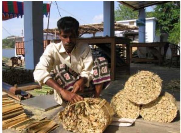
*Converting cylinders into slats (left); bundling of slats (right)*
